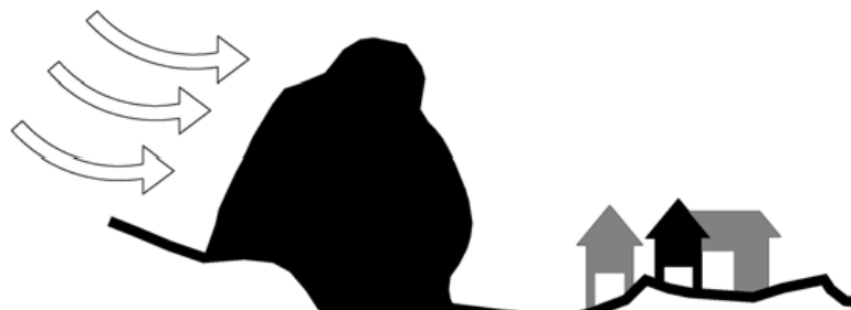
Shielding of house by hillock
