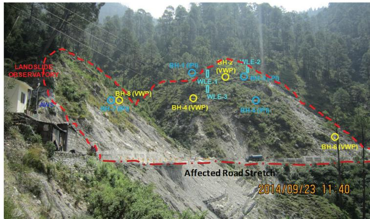
**Figure 8.** Pakhi Landslide selected for instrumentation and real-time monitoring (BH – Bore hole; IPI – In place Inclinerometer; VWP – Vibrating Wire Piezometer; WLE – Wire Line Extensometer; AWS – Automatic Weather Station)
