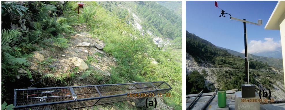
Figure 10. (a) Wire-line extensometer (WLE); (b) Automatic Weather Station (AWS)
