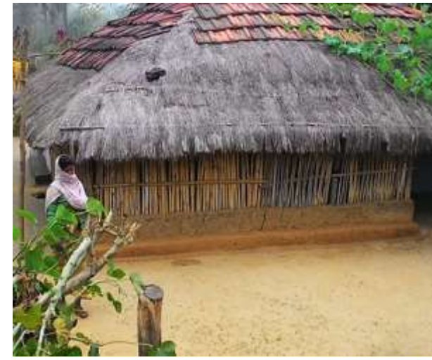
Wattle and daub walls with thatch/tilled hipped roof - Jharkhand
