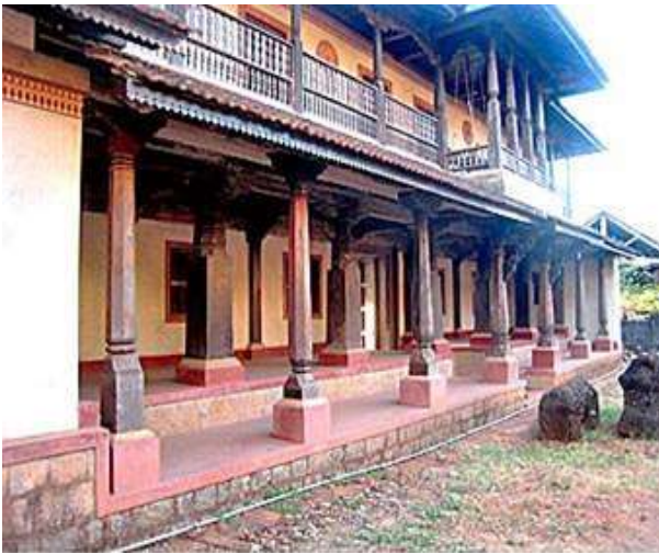
Ashlar Stone Walls with Mangalore tiles gabled roof- Karnataka
